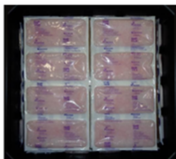
Step 4. Place two room temperature PCM assemblies side by side and centered evenly on top of the product box. Ensure that the 17C/orange side is facing the product box.
