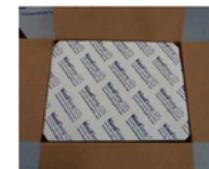
Step 8: Place the PUR lid on top of the PUR base. Close and seal the outer corrugate container using packing tape
