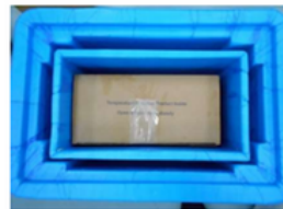
Step 3: Place approx. 5.0 lbs. of pelletized dry ice (not shown) on top of the product box. Fill the left and right cavities between the PUR inner box and PUR base each with approx. 3.0 lbs of pelletized dry ice (not shown) and fill the front and back cavities between the PUR inner box and the PUR base each with approx. 5.0 lbs of pelletized dry ice (not shown), approx. 16.0 lbs. total.
