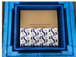
Step 2: Place two refrigerated 722G14+3C PCM gels each side by side evenly folded around the front and top sides of the product box.
