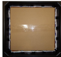
Step 3. Place one room temperature PCM assembly along the back, front, left, and right sides of the product box (four total). Ensure that the 17C/orange side is facing the product box.
