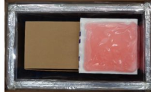
Step 3. Place one room temperature PCM assembly, ensuring the 17C/orange side is facing the product box, with one segment at the right side. Fold down the remaining segment on top of the product box. Repeat on the left side (not shown).
