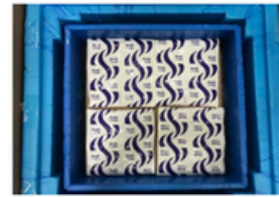
Step 4: Place two refrigerated PCM gels each side by side evenly folded around the back and top sides of the product box.
