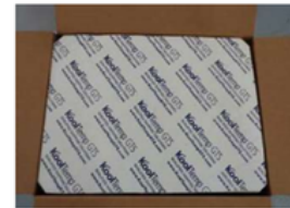
Step 4: Place the molded PUR lid on top of the molded PUR base. Close and seal the outer corrugate container using packing tape
