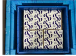
Step 3: Place two refrigerated PCM gels each side by side evenly folded around the back and top sides of the product box.
