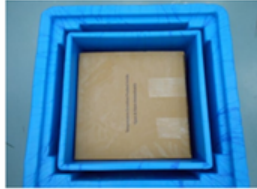
Step 2: Fill the open cavities between the product box and PUR inner box with approx. 25.0 lbs. of pelletized dry ice (not shown).
